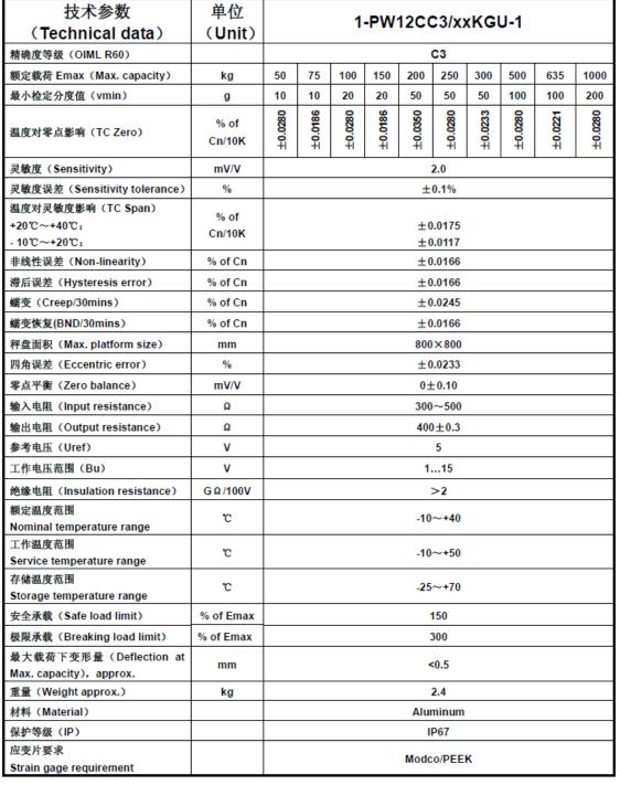
1) The sum of data for Non-linearity, Hystersis error and TC Span meets the requirement of OIML 60
